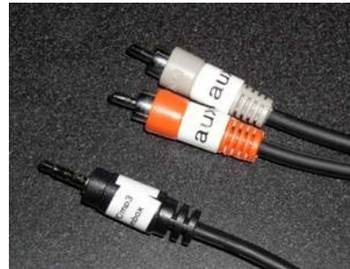
Device patch cables with labels
